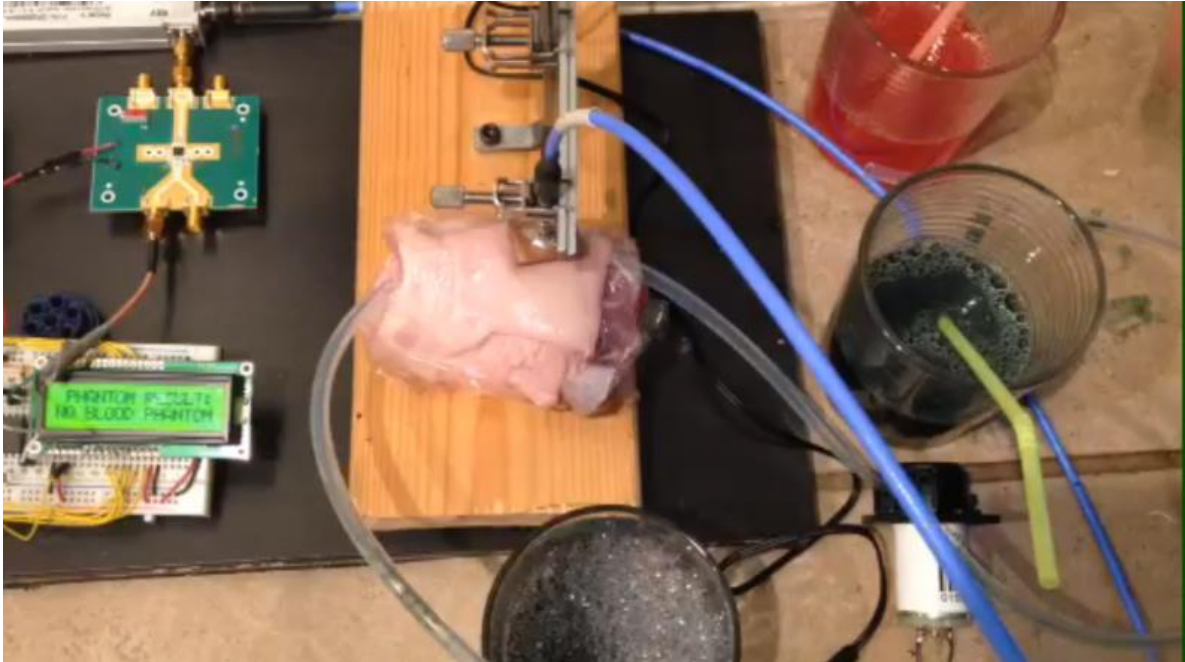
Figure 85: Photograph of the evaluation prototype for non-invasive glucose sensing under test using pork tissue and mimicking liquid blood phantoms.
